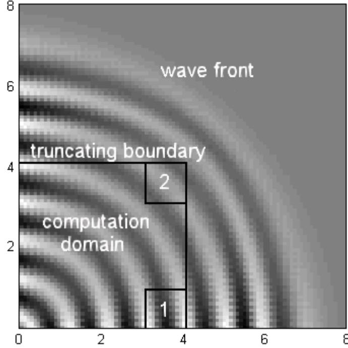
Figure 1 Study ABC performance through radiation of a point source. The unit is meter.
