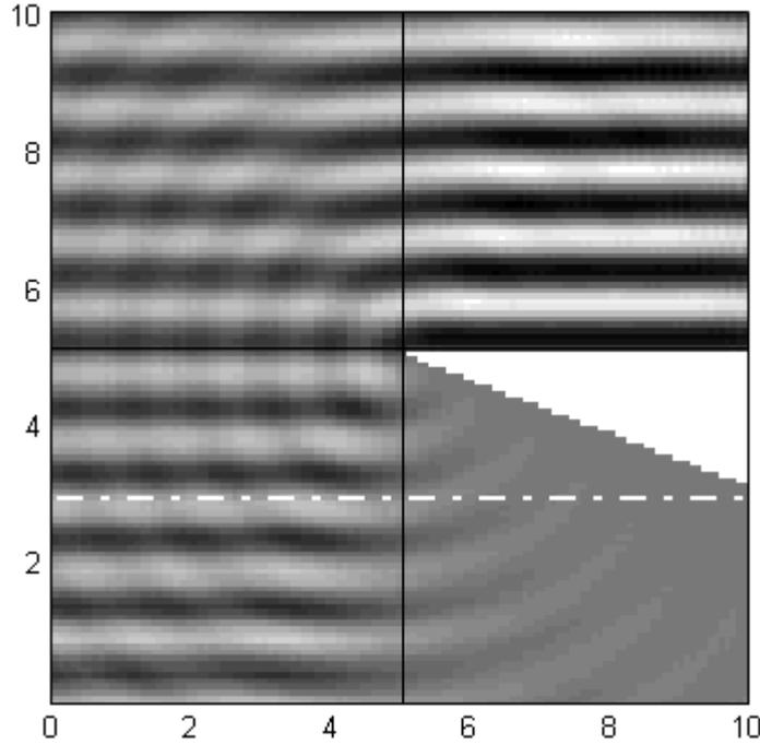
Figure 2 Diffraction of an ideally soft wedge. The vertex angle of the wedge is  $21^\circ$ . The wavelength of the incident sound wave is 1m. The pressure-magnitude distribution on the dash-dotted line behind the wedge and 2m from the insonified surface is illustrated in Figure 3.
