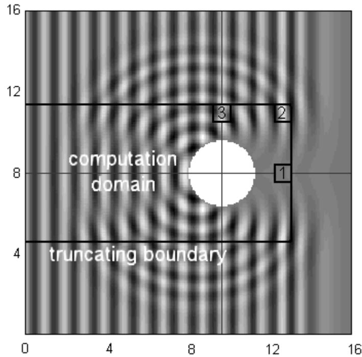
(a) Instantaneous distribution of the total acoustic pressure around the cylinder.
