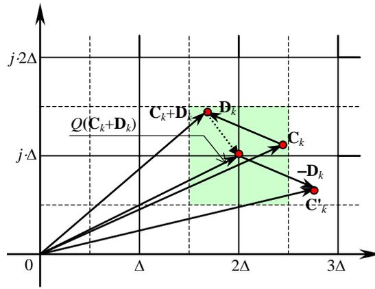
Fig.3 Dither modulation based on Equations (3)~(5). The original complex coefficient  $C_k$  has been modified to  $C'_k$ .
