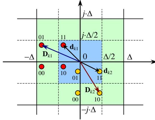
Fig.2 Complex dither vectors  $\mathbf{D}_{k1}$  and  $\mathbf{D}_{k2}$  derived from randomly chosen complex dither values  $\mathbf{d}_{k1}$  and  $\mathbf{d}_{k2}$  based on the doublets to be embedded, which are 01 and 10 respectively.
