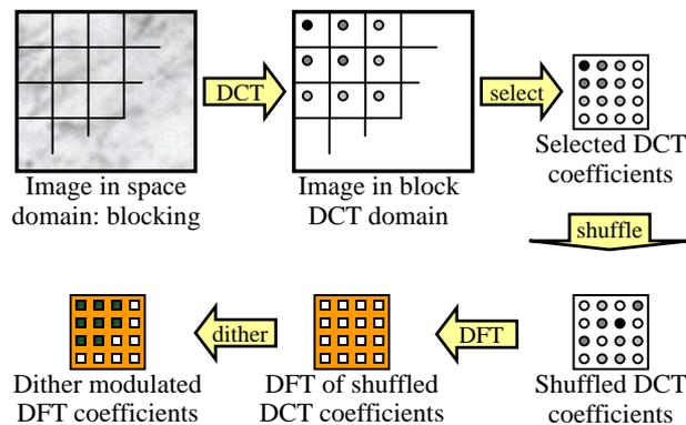
Figure 5 Dither modulation in dual-transform domain
