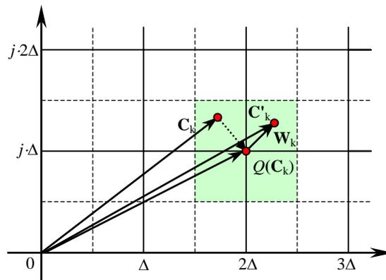
Fig.4 Alternative scheme of QIM in which the host coefficient is quantized and then combined with a coded watermark symbol.
