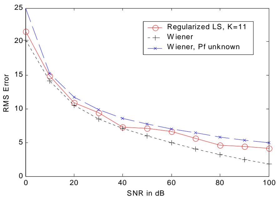
Fig.4 Comparison between LS mask and Wiener filter
