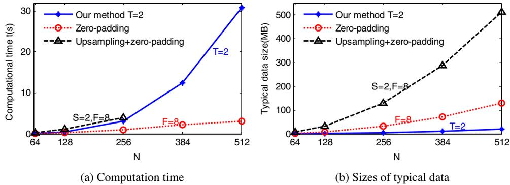
**Fig. 13.** Comparison of computation cost between the proposed method and zero-padding/up-sampling 2D-FFT.
