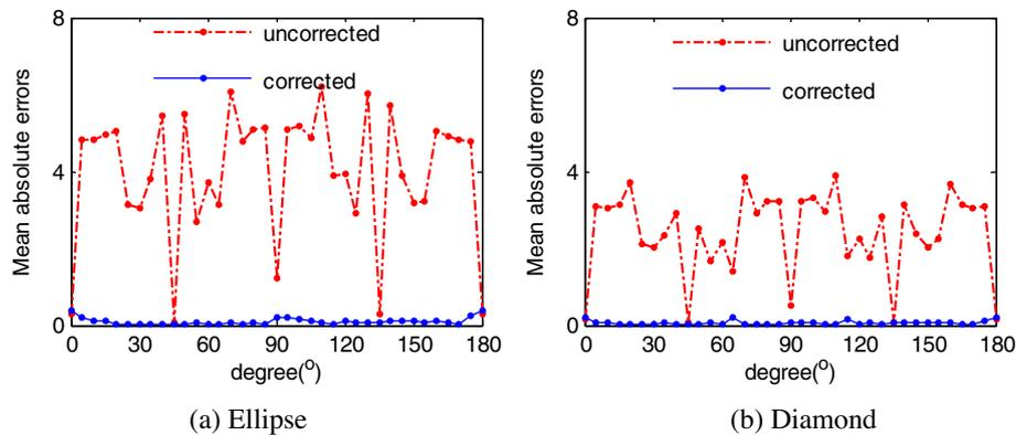
**Fig. 11.** Mean absolute errors of each view. Each plot obtained by mean absolute errors of reconstructed projections from the uncorrected spectrum using the direct 2D-FFT method and the proposed method, respectively.
