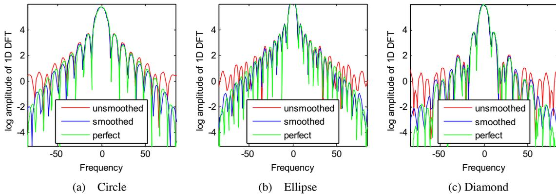
Fig. 5. Comparison of 1D FFT from the original unsmoothed, smoothed, and perfect Radon projections of different objects, with a sound wave incident at 40°.
