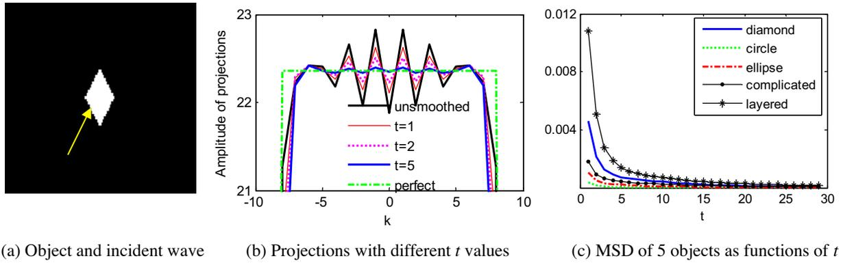
**Fig. 2.** Smoothed Radon projections obtained with different numbers of repeated operations. The wavelength  $\lambda = 1$  m, and spatial sampling interval = 0.1 m. In (c), five objects of different shapes are considered, including one with a more complicated shape and another having a layered structure (see Fig. 10).
