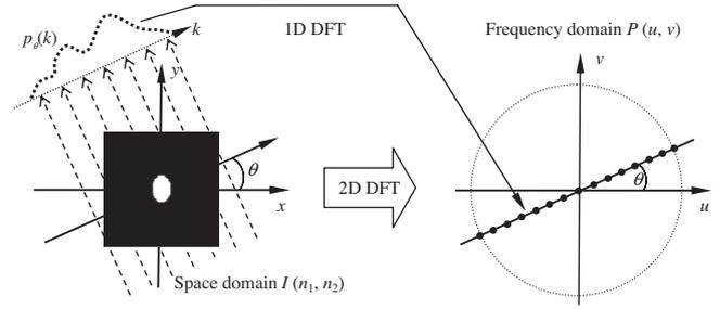
Fig. 1. Radon projection and Fourier slice theorem.
