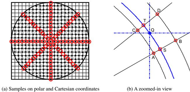
Fig. 6. Interpolation in the 2D Fourier transform domain.
