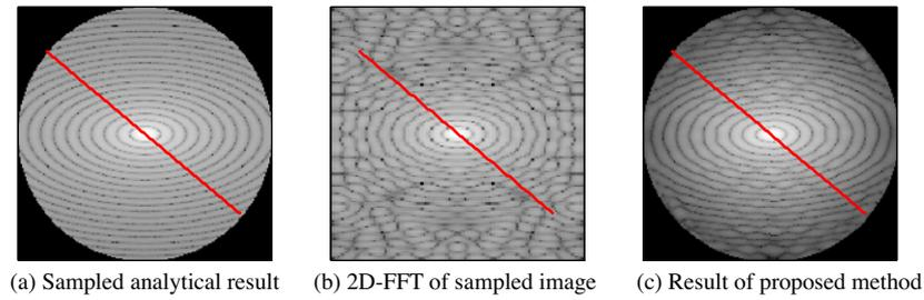
Fig. 7. Spectral magnitude of an elliptical cross-section image.
