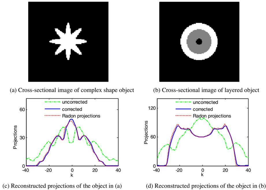
**Fig. 10.** Reconstructed projections of more complicated objects in the direction of  $40^\circ$ . Each of the plots in (c) and (d) contains three curves obtained from the uncorrected spectrum resulted from direct 2D-FFT and the proposed method, and Radon projections from smooth objects respectively.
