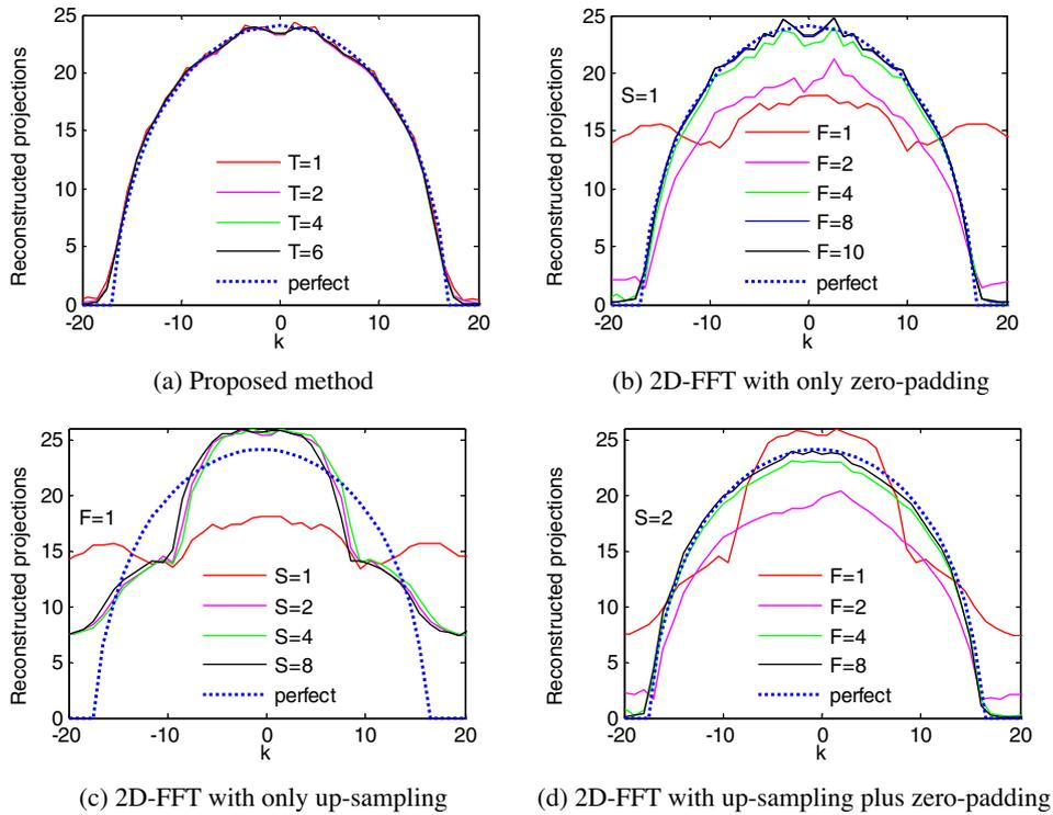
**Fig. 12.** Comparison on accuracy of reconstructed projections.  $T$  is the zero-padding factor in the polar-Cartesian interpolation,  $F$  is the zero-padding factor in 2D-FFT, and  $S$  is the up-sampling factor before 2D-FFT.
