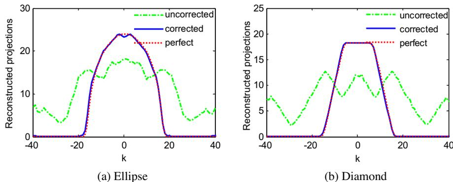
Fig. 9. Comparison of projections reconstructed from the 2D spectrum along  $40^\circ$  along the red lines shown in Figs. 7 and 8. Each plot contains three curves obtained from the uncorrected spectrum resulted from direct 2D-FFT, the spectrum corrected with the proposed method, and the analytically calculated spectrum, respectively.
