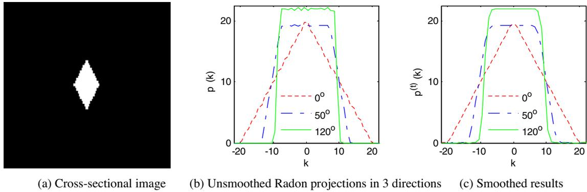
Fig. 4. Comparison between discrete Radon projections and their smoothed versions of a diamond cylinder in water.
