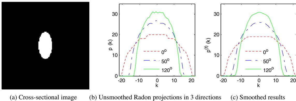
**Fig. 3.** Comparison between discrete Radon projections and their smoothed versions of an elliptical cylinder in water.
